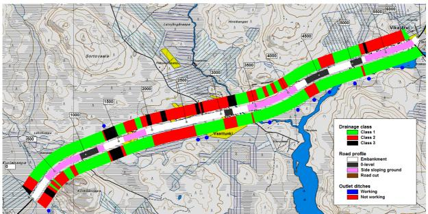
Figure 24. Distribution of the drainage class in section 505. On the left, drainage condition of the left ditch and on the right, drainage condition of the right ditch. Outlet ditches are marked as dots. The road profile is shown in the middle.
