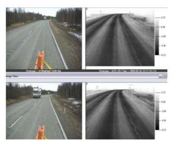
Figure 5. Digital still images and thermal camera images from HW 4, road section 505 in spring 2009. Thermal camera data shows severe top down cracking problems close to the pavement surface. Colder areas in both wheelpaths indicate water pumping through the pavement.
