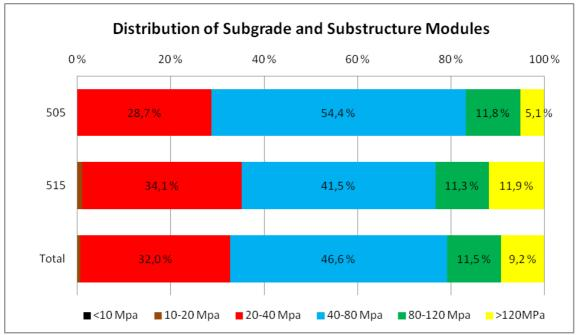
Figure 6. The distribution of subgrade modules in both road sections.
