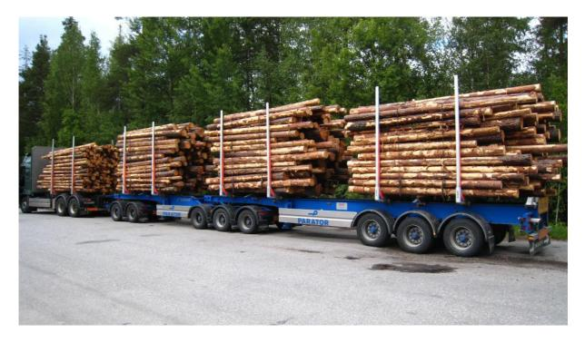
Figure 1. A 30,5 m long and 90 ton heavy truck tested in "En Trave Till" project in Northern Sweden.
