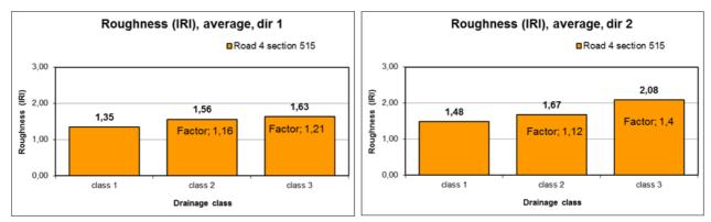
Figure 30. The average IRI values in direction 1 (left) and in direction 2 (right) for each drainage class. The factor inside the column shows how many times larger the value is compared to the value for Class 1.
