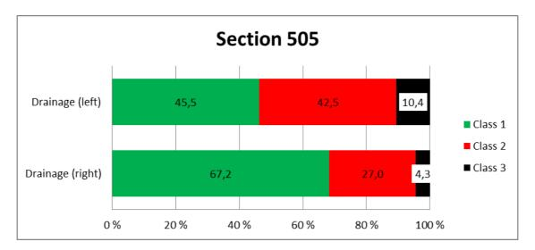
Figure 23. Distributions of drainage class in both ditches of the highway 4 at section 505.
