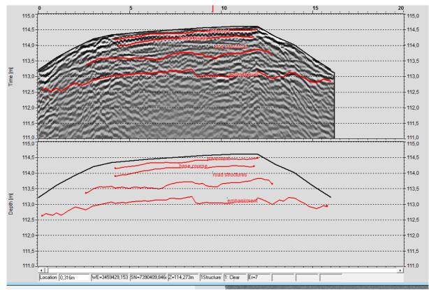
Figure 9. 400 MHz GPR cross section and its interpretation at chainage 3770 m.
