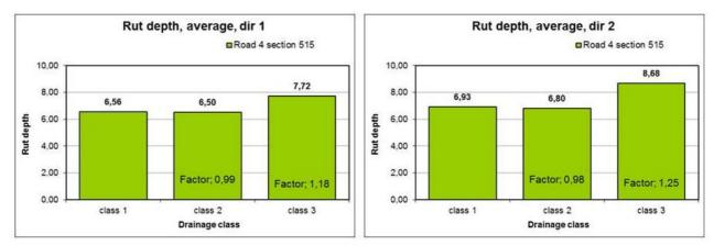
Figure 31. The average rut depth value in direction 1 (left) and in direction 2 (right) for each drainage class.
