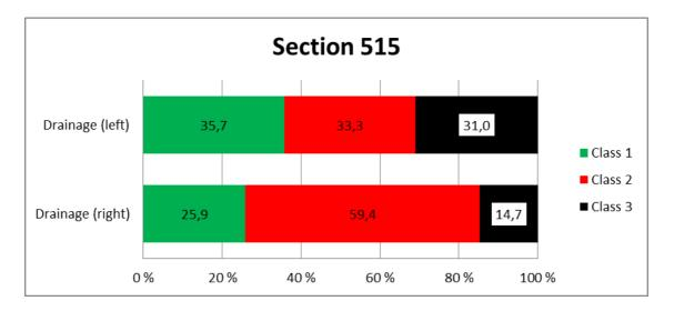
Figure 26. Distributions of drainage class in both ditches of the highway 4 in section 515.
