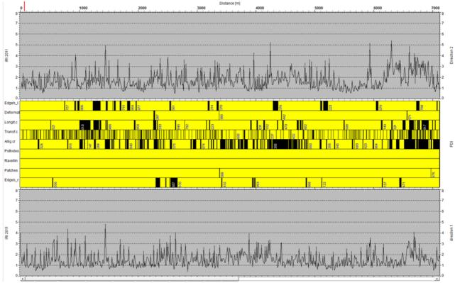
Figure 14. The roughness (IRI, 10 m) values of the right lane (lowest) and left lane (topmost). The pavement distress inventory is shown in the middle.
