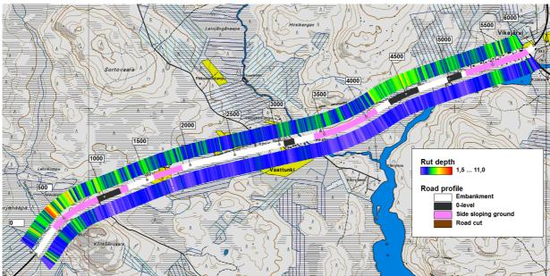
Figure 11. Rut depth in the right lane (direction 1, right) and in the left lane (direction 2, left) in section 505. The road profile is in the middle.
