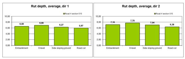
Figure 29. Average rut depth for each road profile in direction 1(left) and in direction 2 (right).
