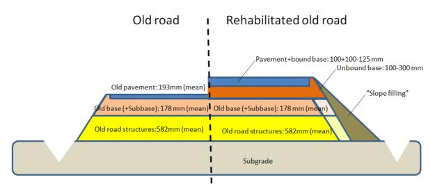
Figure 34. Strengthening structure for risk class section 4 in road section 505.
