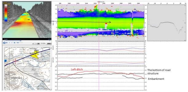
Figure 21. Pole 1050 m. A too shallow left ditch has blocked the flow of water causing frost heaves and transverse cracking in the road. The ditch bottom is higher than the bottom structure of the road and water can flow into road structure. The roughness values have risen in the right lane and the rut depth has started to grow in the left lane. The explanations for data in this figure are the same as for the data in figure 20.
