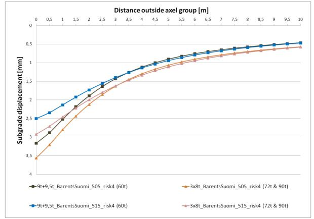
Figure 36. Comparison of the truck options on weak subgrade (modulus 10 MPa) based on the heaviest axle group of each option.
