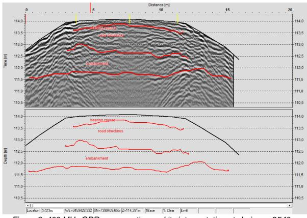
Figure 8. 400 MHz GPR cross section and its interpretation at chainage 2540 m.
