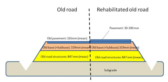
Figure 35. Strengthening structure for risk class section 1-4 in road section 515.
