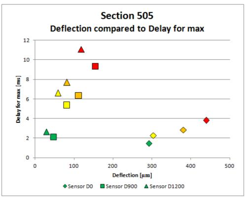
Figure 38. Maximum value of deflection compared to delay for max value on road section 505. Green dots present risk class 1, yellow dots risk class 2, orange dots risk class 3 and red dots risk class 4.
