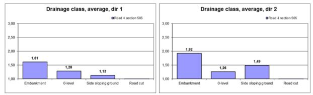
Figure 25. Average drainage for each road profile in direction 1(left) and in direction 2 (right). There were no road cut sections in 505.
