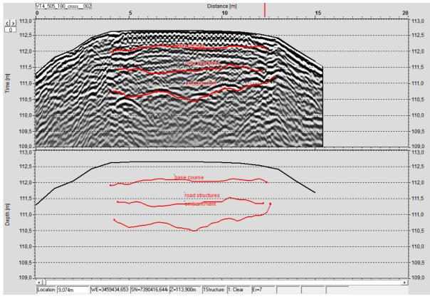
Figure 7. 400 MHz GPR cross section and its interpretation at chainage 180 m.
