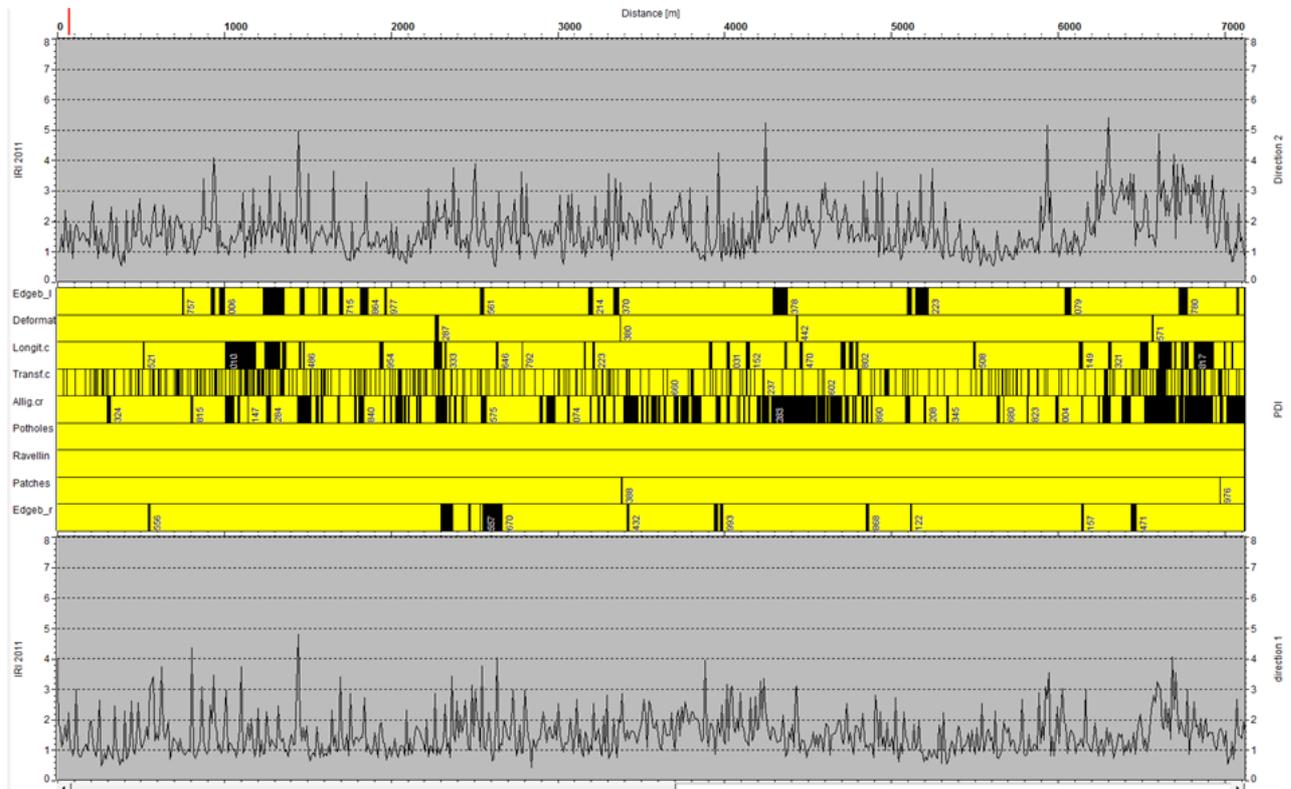
Figure 14. The roughness (IRI, 10 m) values of the right lane (lowest) and left lane (topmost). The pavement distress inventory is shown in the middle.
