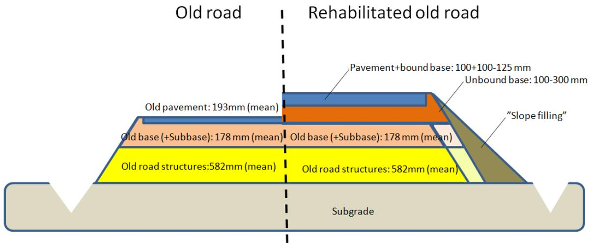
Figure 34. Strengthening structure for risk class section 4 in road section 505.
