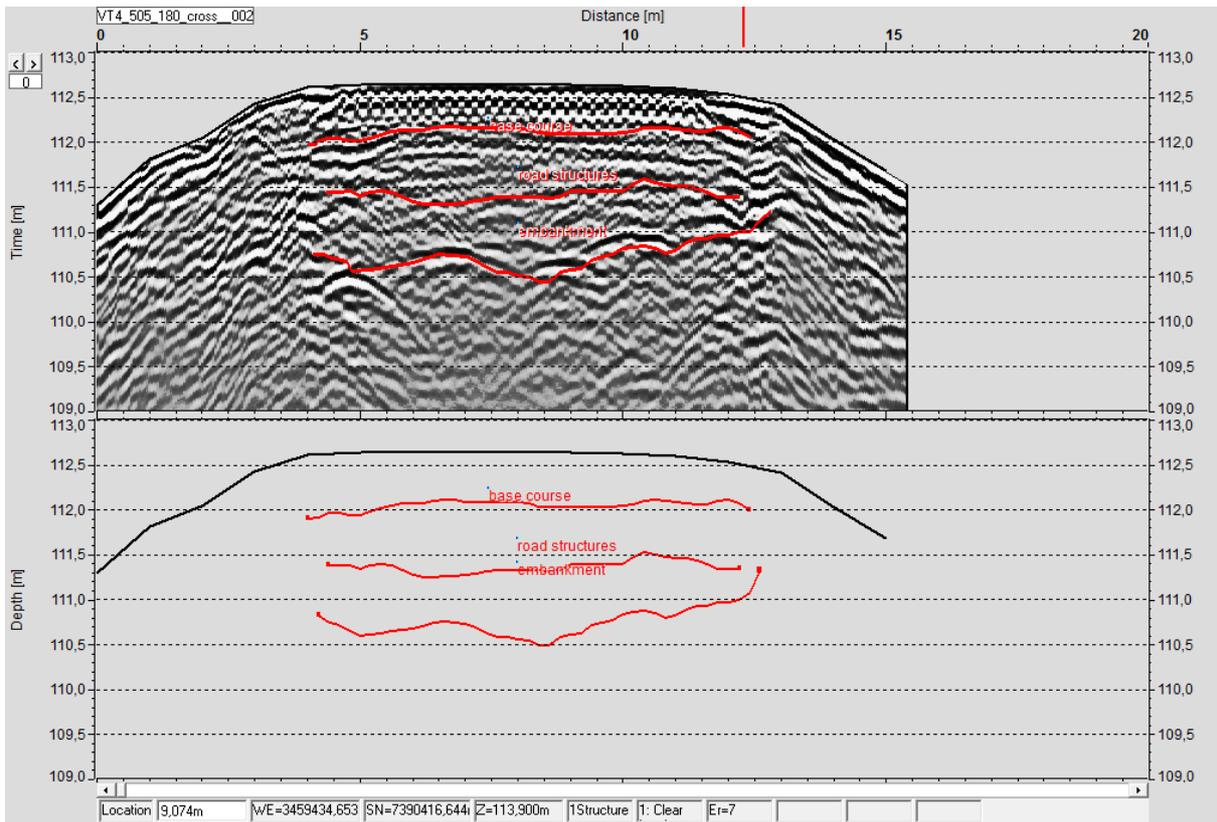
Figure 7. 400 MHz GPR cross section and its interpretation at chainage 180 m.
