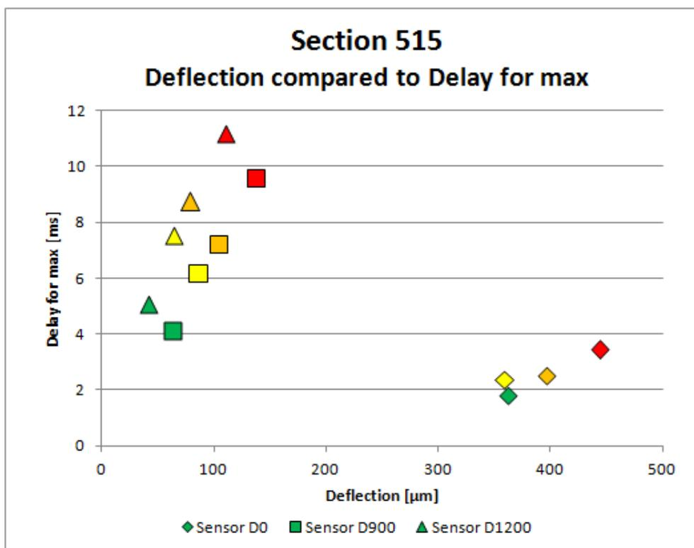
Figure 39. Maximum value of deflection compared to delay for max value in road section 515. Green dots present risk class 1, yellow dots risk class 2, orange dots risk class 3 and red dots risk class 4.
