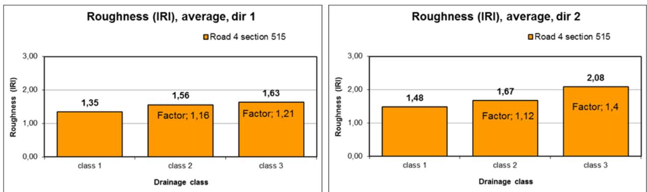
Figure 30. The average IRI values in direction 1 (left) and in direction 2 (right) for each drainage class. The factor inside the column shows how many times larger the value is compared to the value for Class 1.
