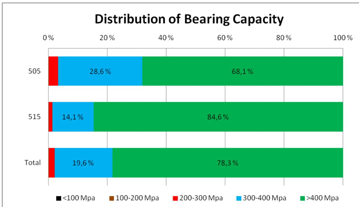
Figure 16. The distribution of bearing capacity in both road sections.
