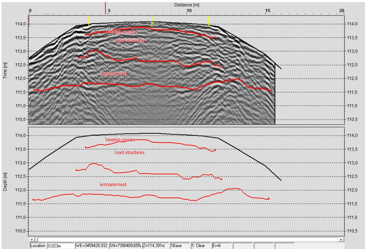
Figure 8. 400 MHz GPR cross section and its interpretation at chainage 2540 m.
