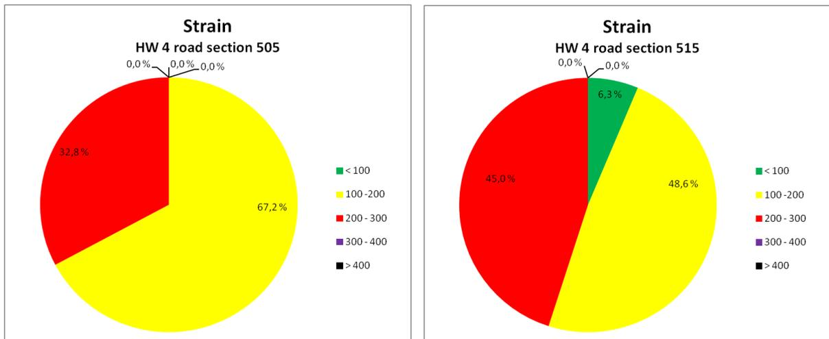
Figure 17. The distribution of strain values in both road sections.
