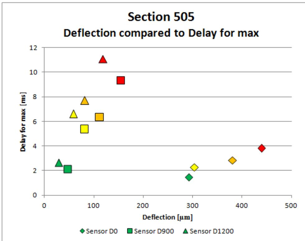
Figure 38. Maximum value of deflection compared to delay for max value on road section 505. Green dots present risk class 1, yellow dots risk class 2, orange dots risk class 3 and red dots risk class 4.
