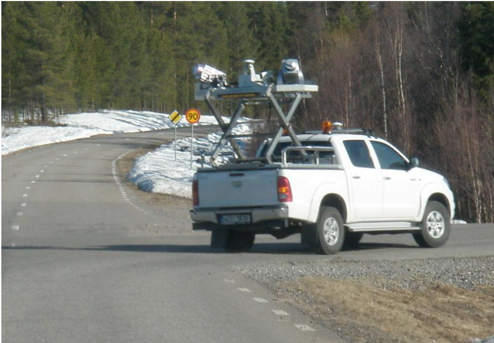
*Figure 3. GEOVAP Quantum 3D mobile laser scanner vehicle in April 2011.*
