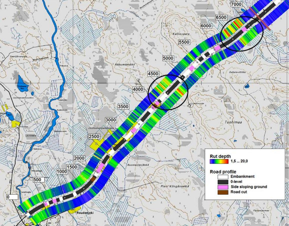
Figure 15. Rut depth in the right lane (direction 1, right) and in the left lane (direction 2, left) in section 515. The road profile is in the middle. The worst places are marked with circles. The supplementary aerodrome begins at the red line.
