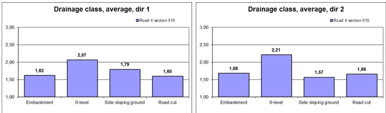
Figure 28. Average drainage for each road profile in direction 1 (left) and in direction 2 (right).
