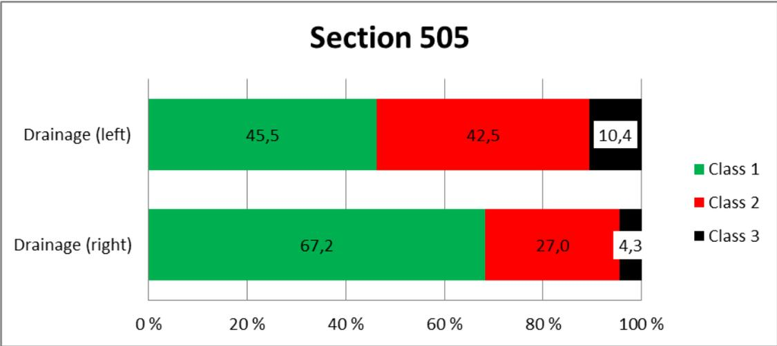
Figure 23. Distributions of drainage class in both ditches of the highway 4 at section 505.
