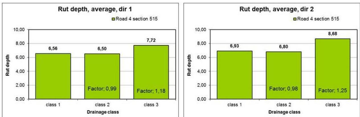
Figure 31. The average rut depth value in direction 1 (left) and in direction 2 (right) for each drainage class.
