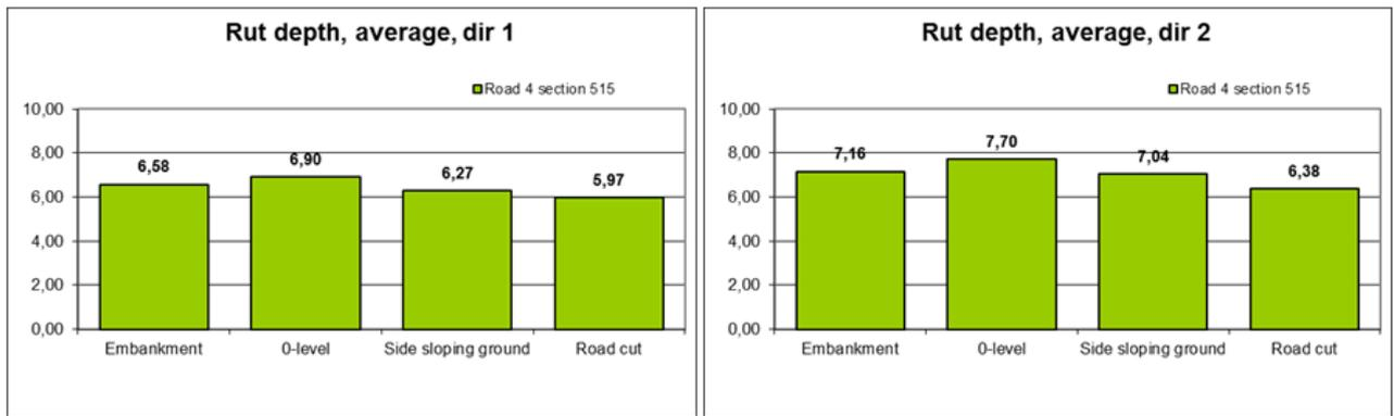
Figure 29. Average rut depth for each road profile in direction 1 (left) and in direction 2 (right).
