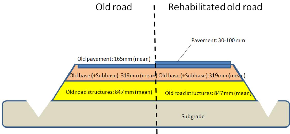
Figure 35. Strengthening structure for risk class section 1-4 in road section 515.
