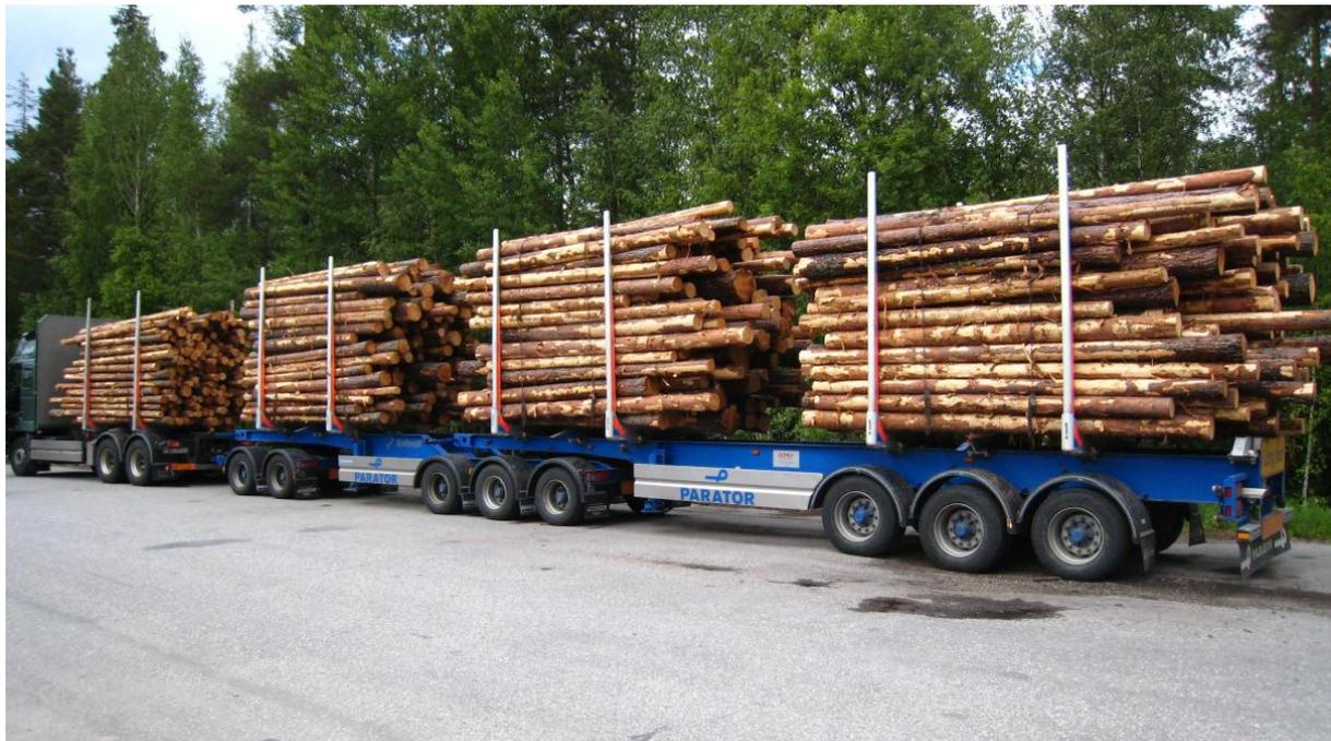
*Figure 1. A 30,5 m long and 90 ton heavy truck tested in “En Trave Till” project in Northern Sweden.*
