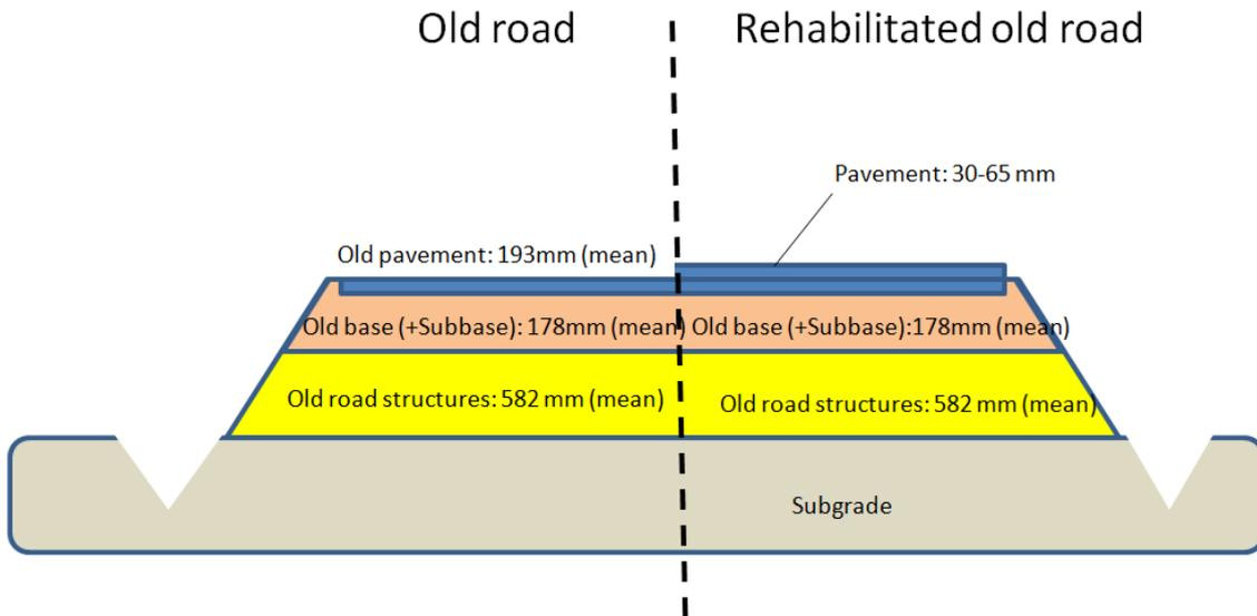
Figure 33. Strengthening structure for risk class sections 1, 2 and 3 in road section 505.
