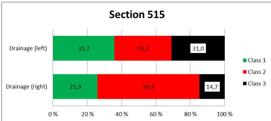
Figure 26. Distributions of drainage class in both ditches of the highway 4 in section 515.
