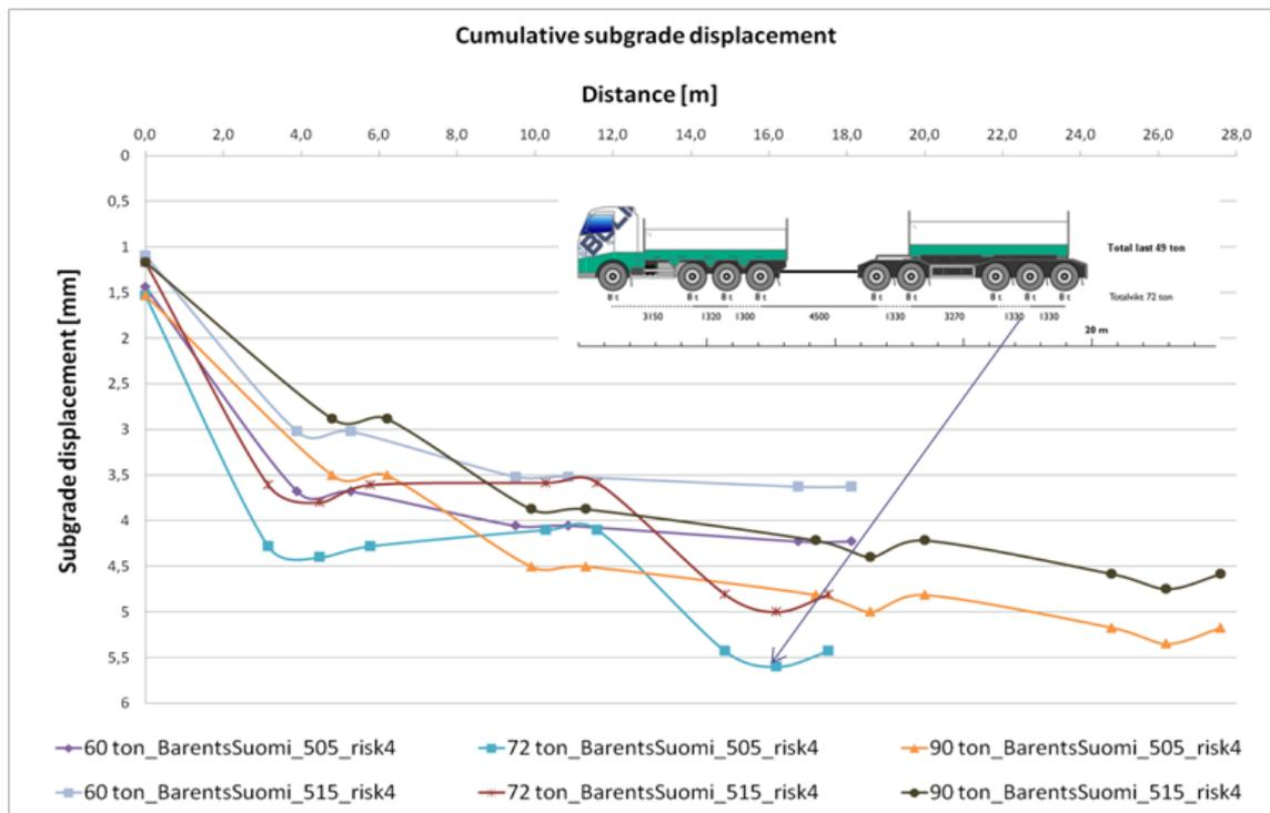
Figure 37. The cumulative displacement of weak subgrade (modulus 10 MPa) calculated for each truck option on both road sections. The horizontal axis presents the distance from the first axle of the truck. Zero is the first axle and the dots along the displacement curve represent the locations of the consecutive axles. On the vertical axis is the cumulative subgrade displacement calculated in one point.
