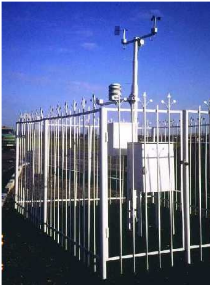
Figure 5-1 A Road Weather Outstation, procured with Tacis-funding, in Ust-Labinsk, in Krasnodar Krai, Southern Russia, protected with light fence.
